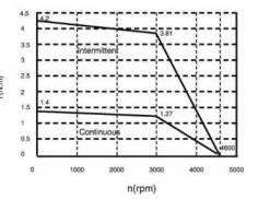
Both motors produce a mechanical / electrical power of 400W at the specified knee on the graph. Both give the same nominal speed and nominal torque.
