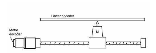
a servo motor is connected to a lead screw through a planetary gear. The load is connected to a secondary linear encoder.
